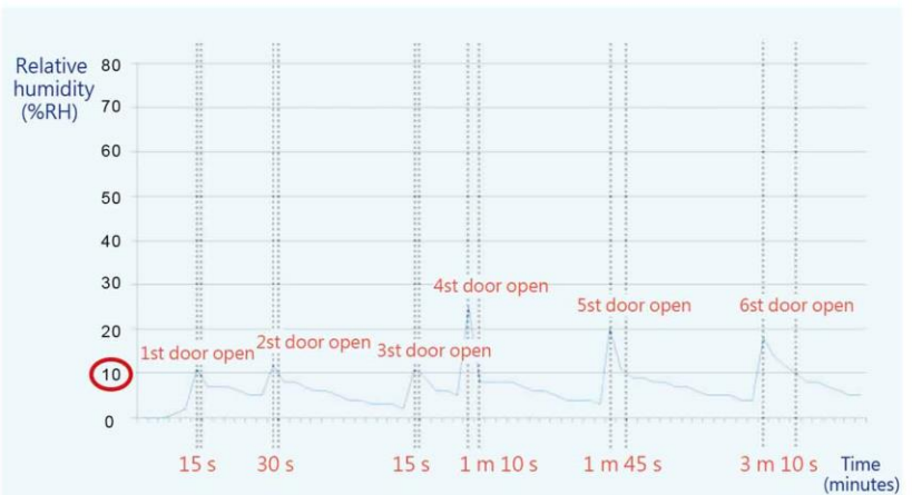
The environment has a humidity of 55%RH, a temperature between 25 to 37 °C, and the test is to open the door for 30 seconds to test the humidity return speed. Depending on external temperature changes, test results may vary.
